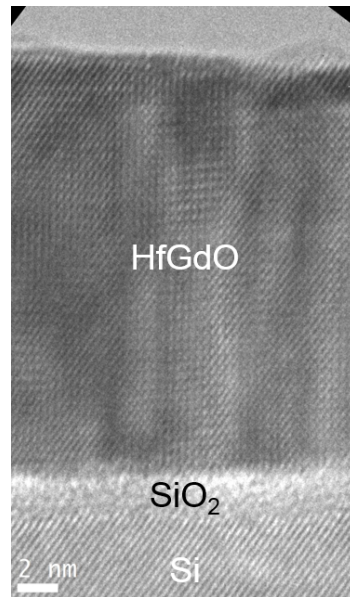
Figure 4.15: TEM image of epitaxial grown HfGdO on Si.
